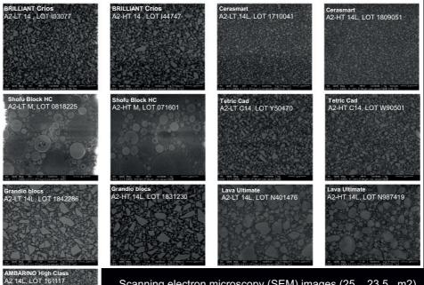
Scanning electron microscopy (SEM) images (25 \_ 23.5 \_m2) of cross sections of the various CAD/CAM RBCs with a constant magnification of 10,000 in BSE mode.
