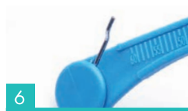
6 Check that the key has reached the stop on the circular end of the handle
