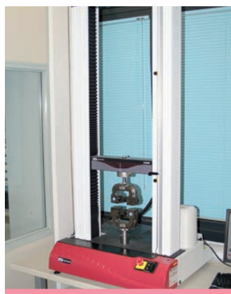
In our Centre for Biotechnological Research "Marco Pozzi", the Shimadzu micro hardness tester and the Instron testing machine are used for the verification of the mechanical properties of the wires.
