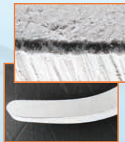
Cutting edge of the Sharp Diamond curette and the magnification of the edge after the test.
